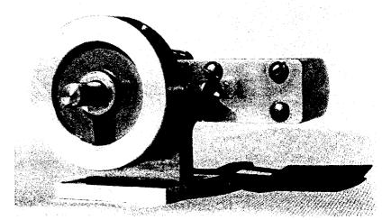
of the Crank set midway between the flats as shown in the assembly view. The Piston is halfway in its stroke and getting full steam. Attach the Crank Disk to the Shaft with a press fit or Loctite.
